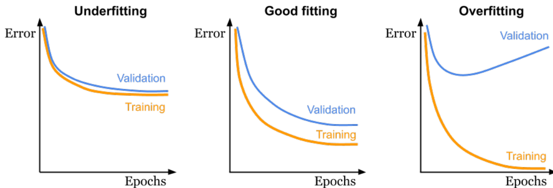
Figure 9.6: Monitoring training and validation losses during model training. The plot illustrates three typical learning behaviours: underfitting (both losses remain high and similar), good fitting (both losses decrease, with validation loss slightly higher), and overfitting (training loss continues to decrease while validation loss plateaus or increases), highlighting the importance of tracking these metrics to assess model performance and generalisation.
